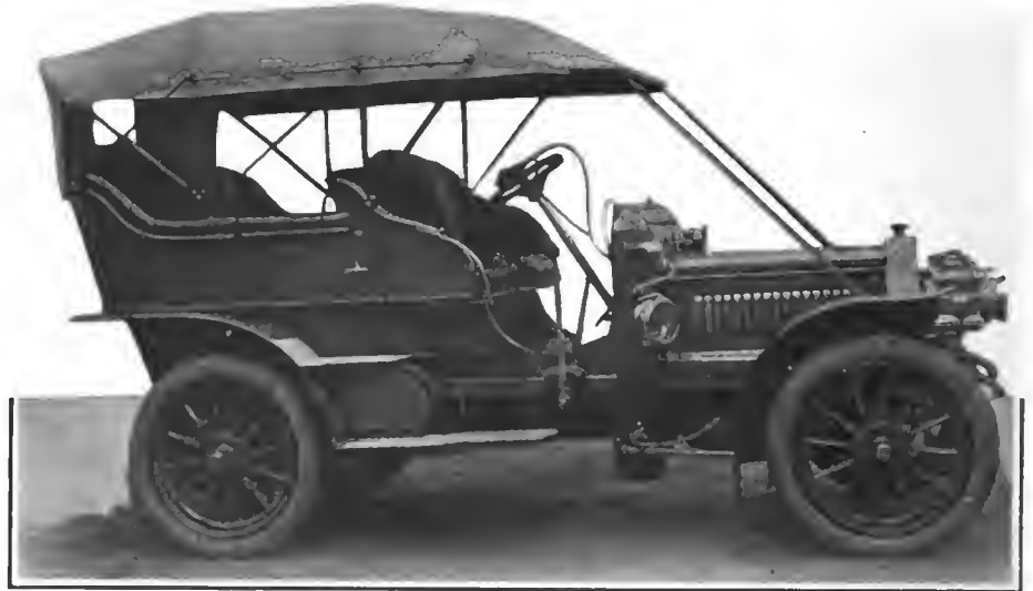
ENGLISH DAIMLER 30-40-HORSEPOWER PHAETON FOR 1906, WITH CAPE CART HOOD.
